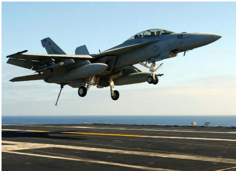
An F/A-18 Hornet fighter/attack aircraft swoops in for an arrested landing aboard the carrier John C. Stennis off the California coast (USN photo)
